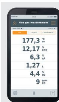
The operation of the measuring instrument as well as the display of the measurement values take place by Bluetooth via the testo 330i App on your Smartphone or tablet – independently of the measurement location. In addition to this, you can use the App to create measurement reports, add photos and comments to these, and send them by e-mail. For iOS and Android.
